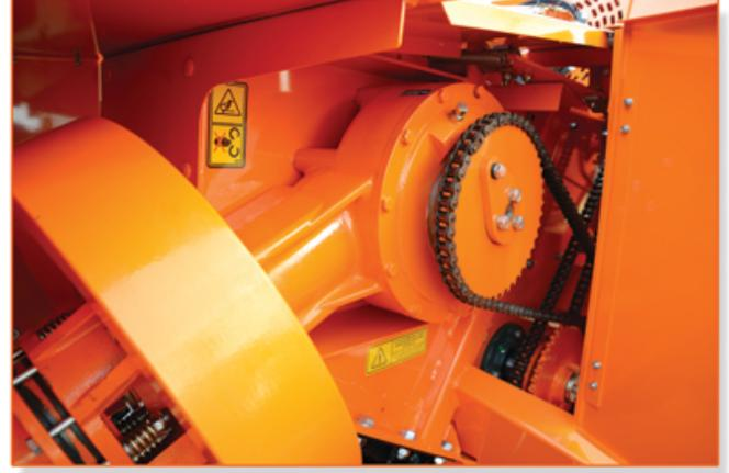
120 rpm transmission gear provides sturdiness, knockless and smooth operation.
