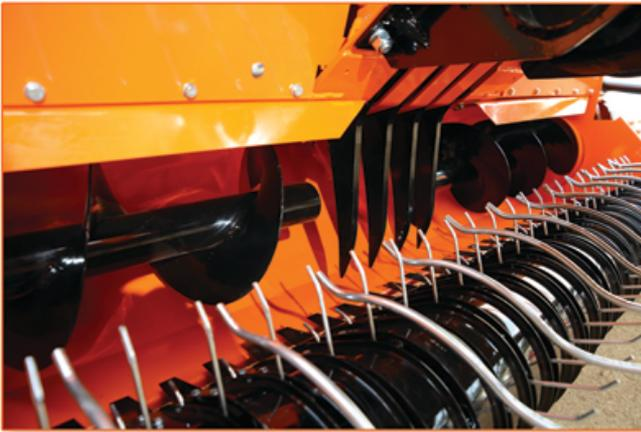
Crank feeder system provides the highest level of product flow with high-strength spiral and special design.
