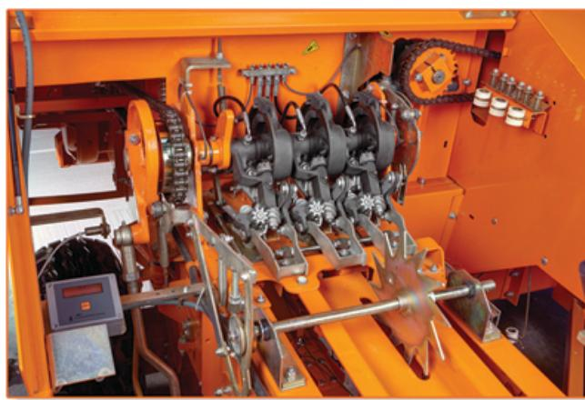
*2 twines / 3 twines knotter set works flawlessly and high-accuracy with its central lubricating system*
