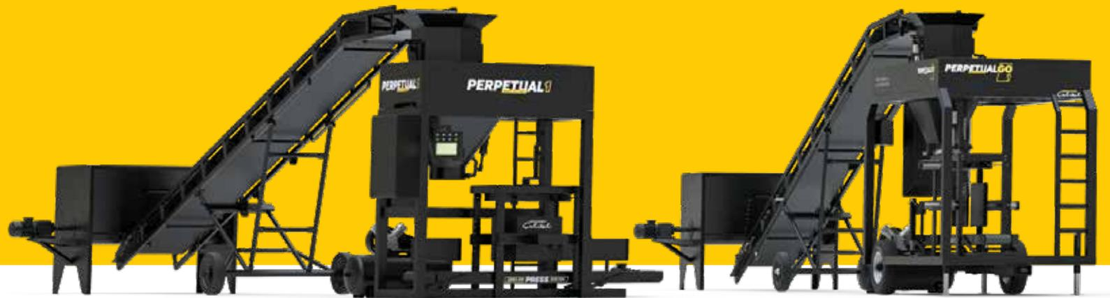
PERPETUAL® packaging concept begins with the transfer of materials prepared by a mixer onto a band. Materials delivered to the dispensing system via the band are transferred from here into bags. After the air is removed from the package, the movement of material in the system ends by pressing and closing the top of the bag. Since the pressing process is the main factor in the life of the packaged product, the pressing process will be ideal thanks to the four powerful pneumatic piston.
